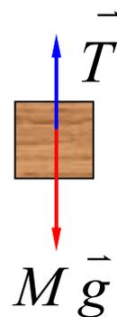
**A**  $\left\{ \begin{array}{l} Tr = J\alpha_A = J\frac{a_A}{r} \\ Mg - T = Ma_A \end{array} \right.$
