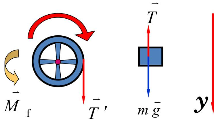
$$\left\{ \begin{array}{l} m_1 g - T_1 = m_1 a_1 \\ T_1 R - M_f = J \frac{a_1}{R} \\ h = \frac{1}{2} a_1 t_1^2 \end{array} \right.$$
